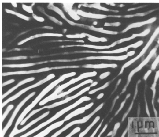
Figure 9 Micrograph showing the two-phase lamellar structure after cooling to room temperature.
