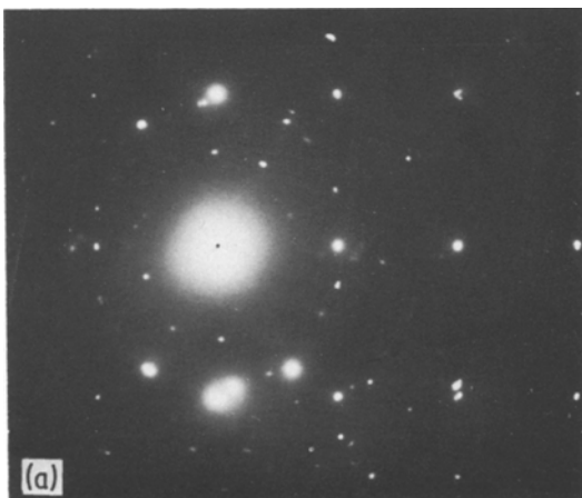
Figure 12 Typical diffraction patterns from the two-phase structures.
