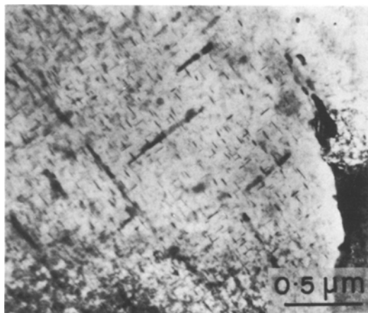
Figure 7 Micrograph showing a high density of Widmanstätten type of precipitates when the foil is annealed at 623 K for 30 ksec.
